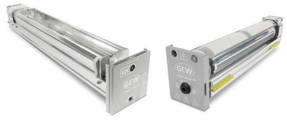
E2C & VCP\* cassettes are designed and manufactured for the harshest environment with optically tuned reflectors to maximise the lamps' curing effect. To maintain the long-term operation of the UV system the cassettes should be serviced regularly (every two years). The service can increase the output of the cassette by up to 90%.
