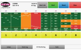
UV intensities for each lamp can be displayed in graphical or tabular form. Traffic light colouring warns when a lamp is approaching or exceeding set points.
